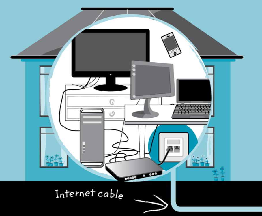
Usually your home is connected to the internet by a wire that is buried in the ground to a cabinet where many wires are connected to a large internet cable.
